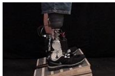
A robotic prosthesis for transtibial amputees
